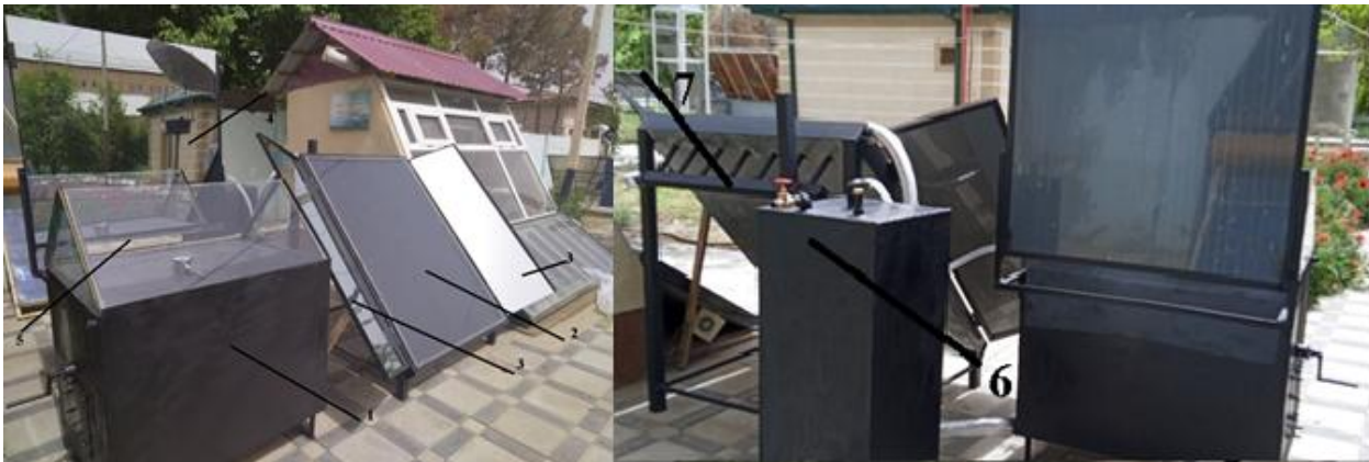
Figure 1. Device for heliothermic treatment of municipal solid waste.
