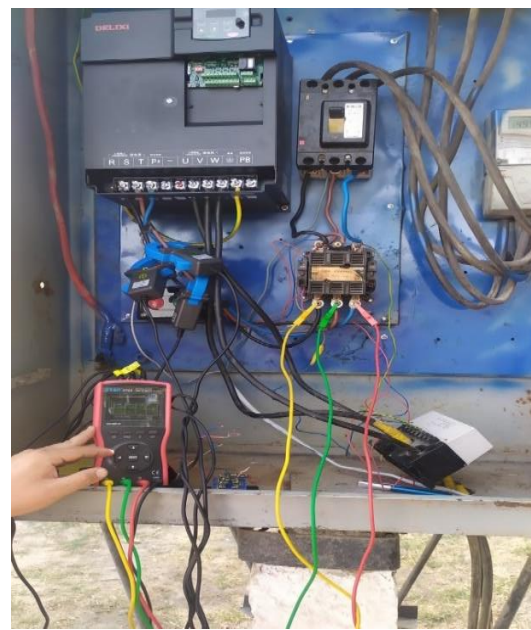
Figure 8. The process of conducting experiments using a built-in frequency converter
