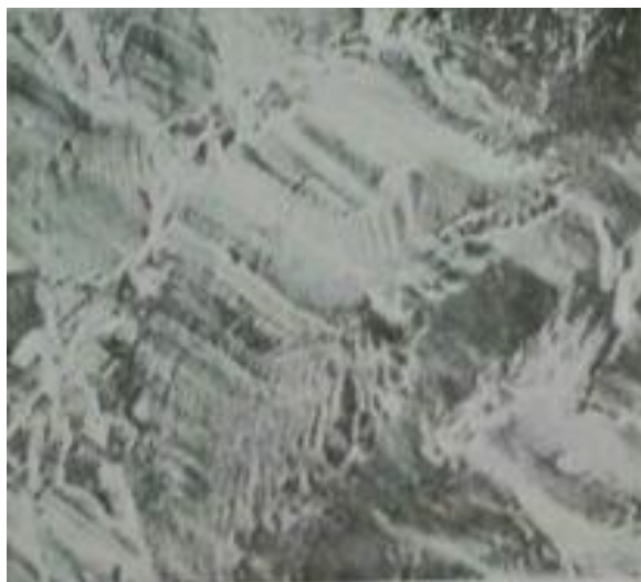
Picture. 2. Fatigue fractogram destruction of metal deposited cored wire PP-Np-08H16B (X320, reduced 2/3)
