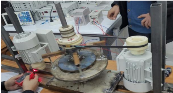
Fig. 7. Axial flow synchronous generator rotor and stator moved against each other.
