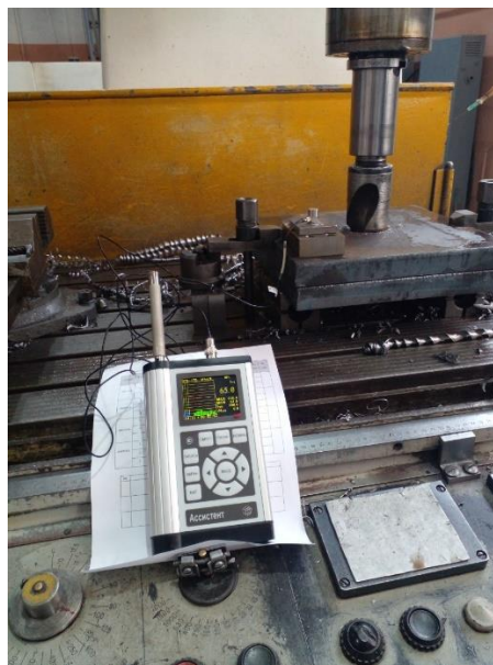
Fig. 3 - installation of sensors on the drill in the analysis of signal stability based on the 2A135 machine: 1 - sensor, 2 - wave converter
