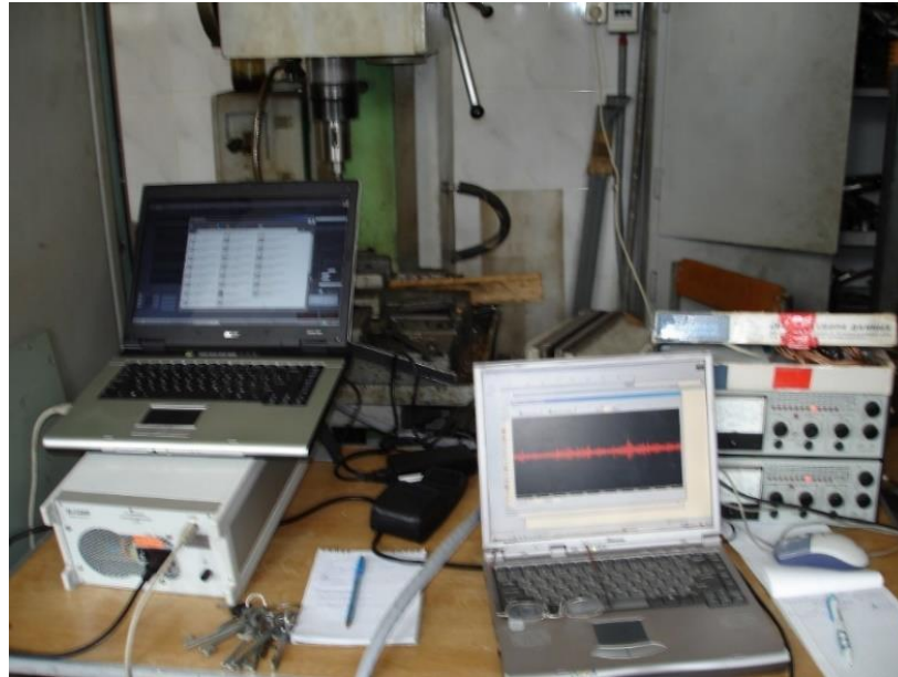
Figure 1 – stability analysis of the vibroacoustic signal based on the 2A135 bench.
