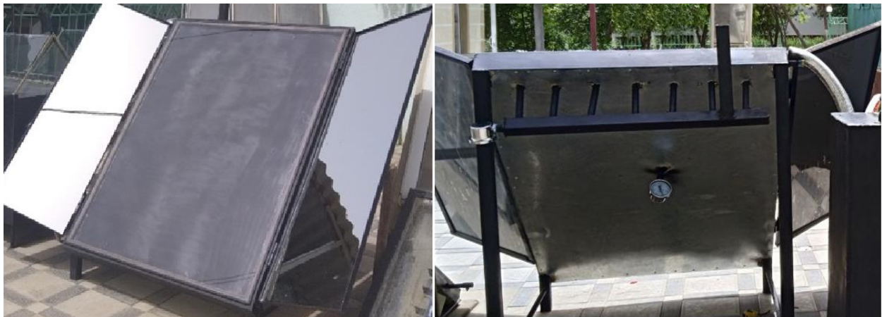
Figure 2. Front and back view of flat reflector solar air heating collector with heat storage.
