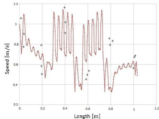
Fig. 8. Change in flue gas velocity in the channel of a hot water boiler unit: — calculation; + experiment.
