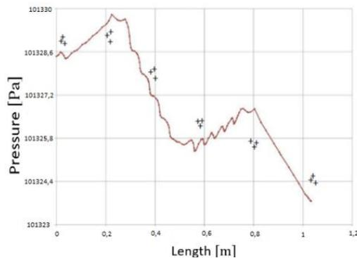
Fig. 7. Change in flue gas pressure in the duct of a hot water boiler unit: — calculation; + experiment.
