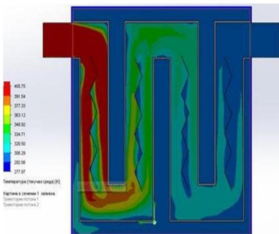
Fig. 4. Temperature change of flue gases in the channel of the local hot water boiler.
