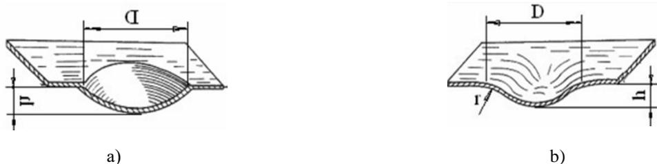
Fig. 2. Constructions with recesses: a) with a sharp edge; b) with a smooth edge; D is the diameter of the recess; h is the height of the recess; r is the radius of the base of the recess.
