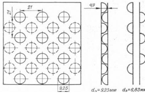
Fig. 3. Chessboard arrangement of depressions on one side and bulges on the other side of the wall of the heat exchanger.
