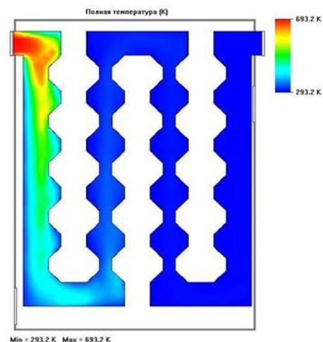
Fig. 5. Change in the temperature field of flue gases in the channel of a local hot water boiler.
