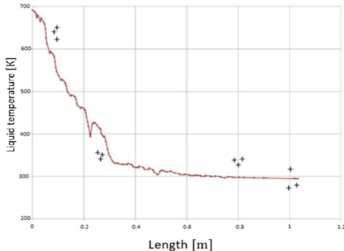
Fig. 6. Temperature change of flue gases in the channel of a hot water boiler unit: — calculation; + experiment
