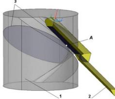
2-picture. The solid models are the 1 organizers and the 2 instrument, and the 3 are their intersection in the plane of the YZ coordinates, a point is the intersection of these
