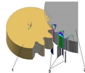
7-picture. Instrument Model (1), organizers (2), as well as clipped layers (3)
