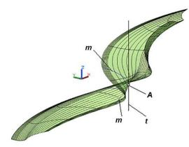
1-picture. The helical surface, its sections m and the plane n, the coordinates ZY and ZX parallel, the intersection of these parts t at point A
