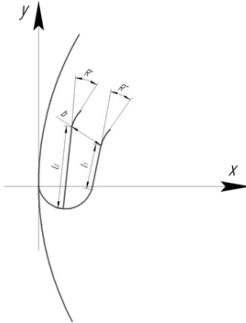
**Figure 1. Scheme of installation of the proposed nozzle on the drum.**
