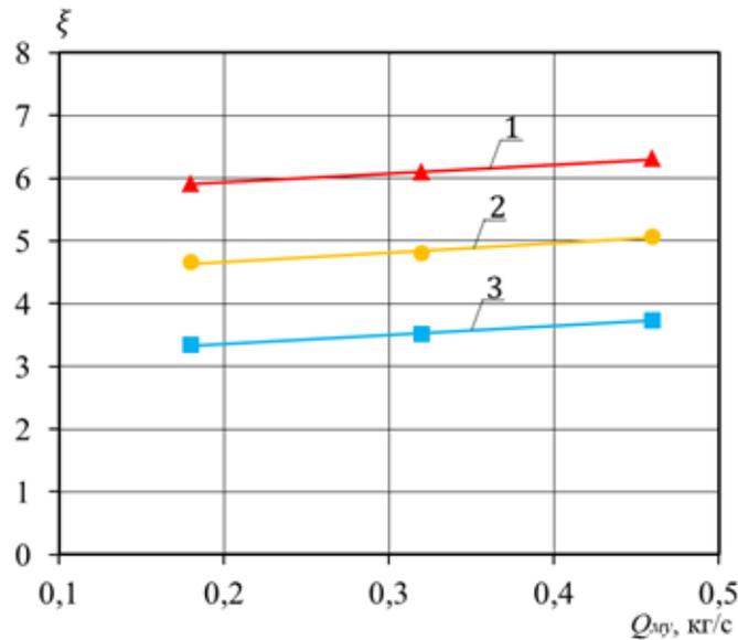
1 working capacity 0.18 kg / h; 2 working productivity 0.32 kg / h; 3 working productivity 0.46 kg / h;
