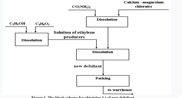
Figure 1. The block scheme for obtaining 1 t of new defoliant
