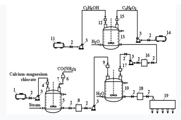
Figure 2. The basic technological scheme for obtaining of new defoliant 1,11,14-storage tanks; 2-valves; 3-centrifugal pumps; 4,9,12,15,17-meters; 6-bins; 7-tape weight dispensers; 5,10,13-reactors; 8,16,18-intermediate tanks; 19-packing.
