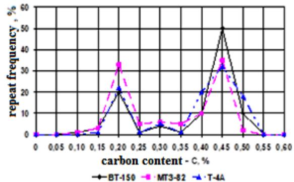
b) distribution of remanufactured parts by the amount of carbon in the material
