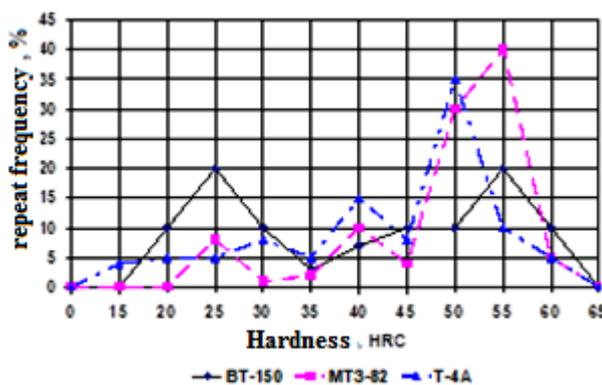
v) distribution of remanufactured parts by metal hardness
