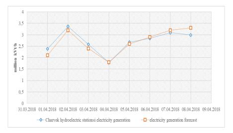
2- figure. Actual and forecast electricity generation calculated on the basis of data on the water supply in the snow april Charvak hydroelectric power station.
