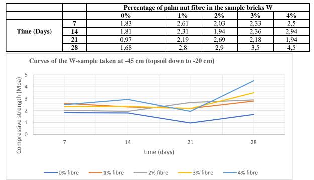
Figure IV.D.d: Compressive strength curves of mud bricks of sample W stabilized with palm nut fibres
