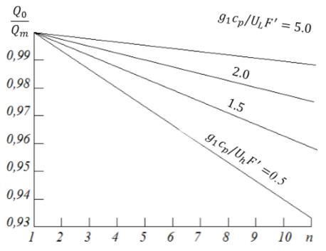
Fig.2.Daily productivity of the collector for signgle-and heating cycles as a function of circulation multiplicity for different values of the parameter  $g_1c_p/U_LF$ `.
