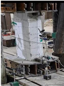
**Fig.6: LVDTs setup.**
