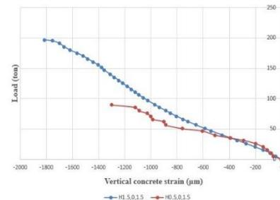
Fig.15: Ultimate load versus Vertical concrete strain.
