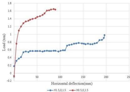
Fig.14: Ultimate load versus horizontal deflection.
