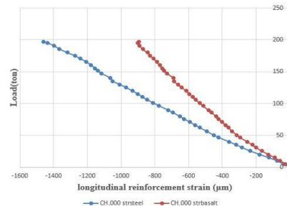
Fig.17: Ultimate load versus longitudinal reinforcement strain column H1.5,0,1.5.
