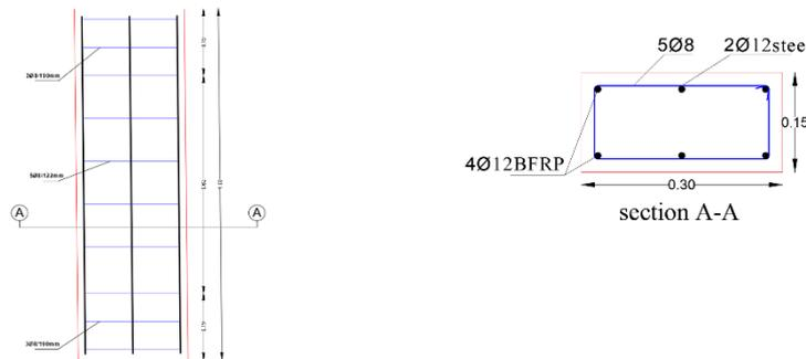
**Fig.3:** Details of specimens.
