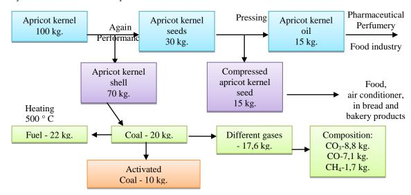
Figure 2. Scheme of complex processing of apricot seeds for material support units
