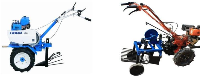
**Figure 1. Motoblocks equipped with excavating working bodies of various constructions**
