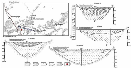
Fig.3. Scheme of location and structure of the Lavlyakan deposit of astrakhanite and halite: 1 - halite; 2 - astrakhanite; 3 - silts; 4 - gypsum; 5 - sand; 6 - observation points.
