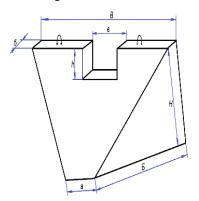
$a = 1 \div 2$  m width of fence bottom, corresponding to width of the collector;
