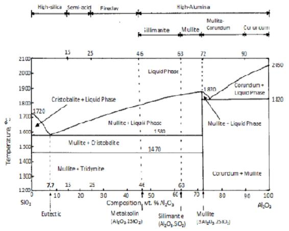
Figure I: SiO<sub>2</sub> – Al<sub>2</sub>O<sub>3</sub> System showing subgroups of aluminosilicate refractories {Adapted from Krivandin and Markov (1980); and Callister (2007)}
