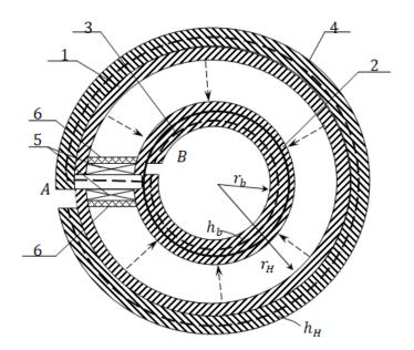
Fig.1. Flow transducer EMR
