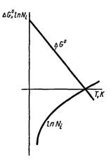
Fig. 2. Dependence  $\Delta G^0$  and logarithm of the pressure of dissociation of metal oxide on temperature
