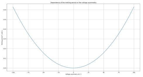
Figure 1. Graph of the relationship between voltage asymmetry and metal melting time
