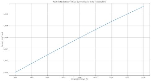
Figure 3. Graph of the relationship between voltage unbalance and metal recovery time
